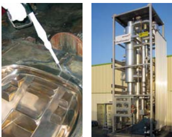
Left: Cleaning with dry ice pellets is increasingly replacing conventional blasting methods.
