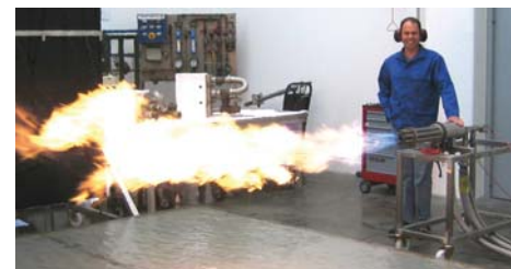
The technical center in Gumpoldskirchen received an enhanced burner test stand.
