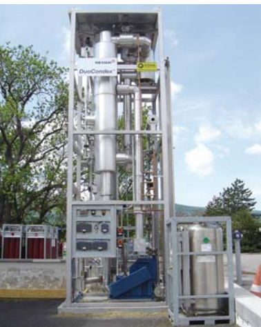
DuoCondex is a process for recycling refrigerators.
