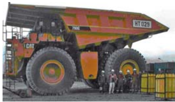
The huge tires of mining trucks are filled with nitrogen.
